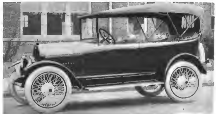
Side view of the Jeffery Roll-Edge Four for 1917, showing the unbroken body lines and the feature which gives the car its name. Wheelbase is 116 in. and tires are 34 by 4. The car sells for $1,095 with complete equipment
